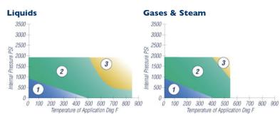
The pressure/temperature graphs shown are the most current method of determining the suitability of a gasket material in a known environment. Use the pressure and temperature graphs to select the most suitable material for your application.
