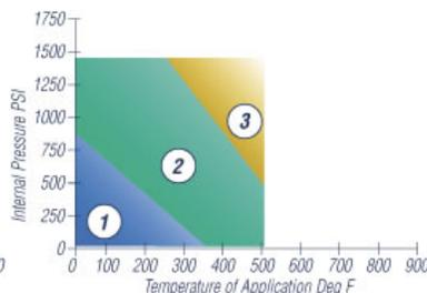
The pressure/temperature graphs shown are the most current method of determining the suitability of a gasket material in a known environment. Use the pressure and temperature graphs to select the most suitable material for your application.
