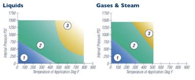
The pressure/temperature graphs shown are the most current method of determining the suitability of a gasket material in a known environment. Use the pressure and temperature graphs to select the most suitable material for your application.
